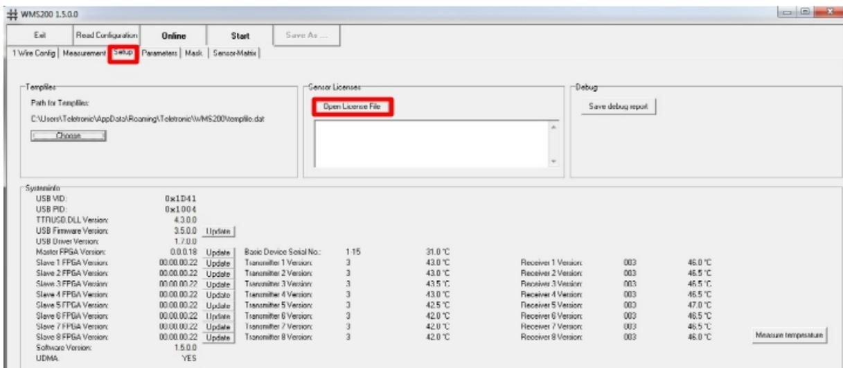
Choose the wsl-file which was delivered with the sensor. From now measurements are possible.
