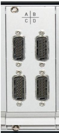
The IO card contains 4 sockets for the receiver modules. The sockets are named with A to D. The sockets on the left IO card used for receiver modules 1 to 4 and the right IO card for receivers 5 to 8.
