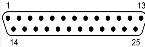
Image 3.6: WMS200 receiving module input plug
