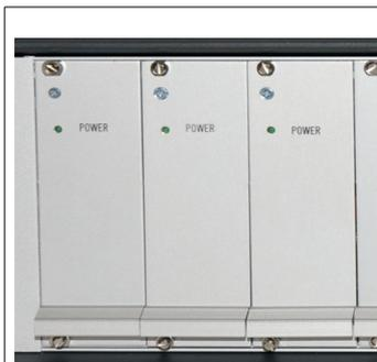
Each power card contains a switching power supply. The green LED should light during normal operation. If not maybe a fuse a is burned out. The right fuse parameters are printed inside the card.
