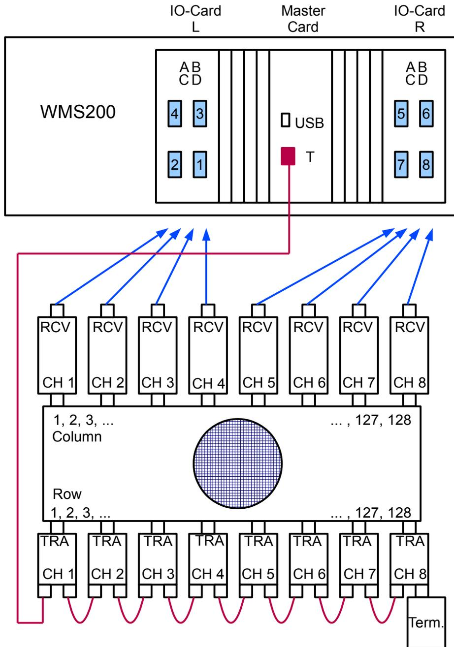
Image 3.7: Cabling plan for a 128 x 128 Sensor
