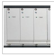
Each power card contains a switching power supply. The green LED should light during normal operation. If not maybe a fuse a is burned out. The right fuse parameters are printed inside the card.
