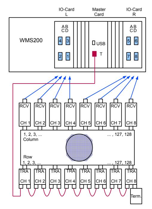
Image 3.7: Cabling plan for a 128 x 128 Sensor
