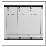
Each power card contains a switching power supply. The green LED should light during normal operation. If not maybe a fuse a is burned out. The right fuse parameters are printed inside the card.
