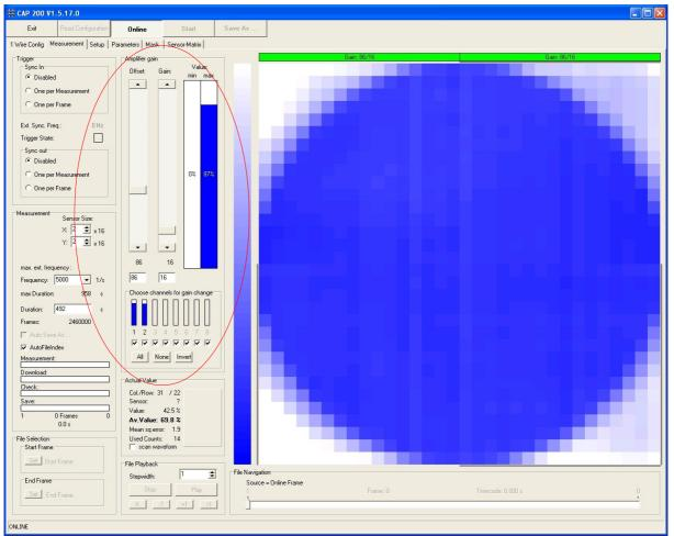
Image 4.4: Offset and gain adjustment
